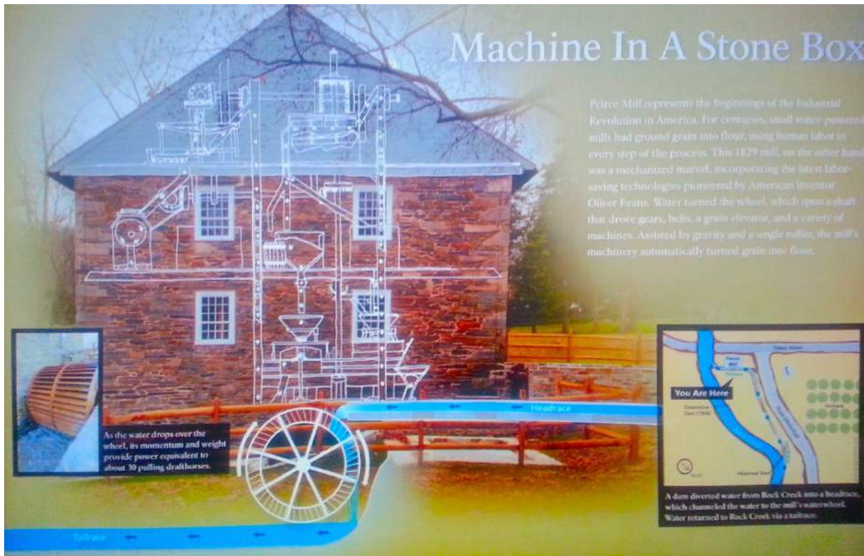
Interior diagram of Isaac Peirce Mill showing early industrial mechanization.
