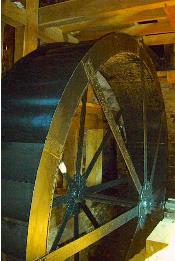
Anselma Mill overshot steel waterwheel (1906) similar to Roxbury Mill wheel (1917) at right.
