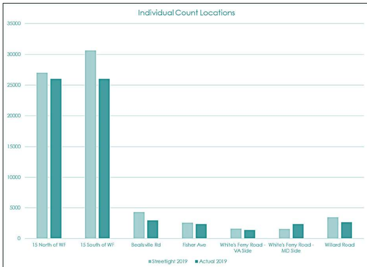
Figure 3-5: Comparison of Estimated and Observed Traffic Counts at Specific Locations
